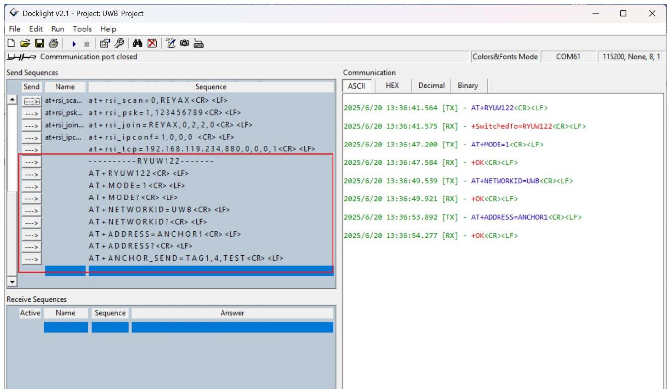
\*RYUW122 is the UWB module used in the RYUW122\_ANCHOR1. For the detailed command set, please refer to the following link for more details:
