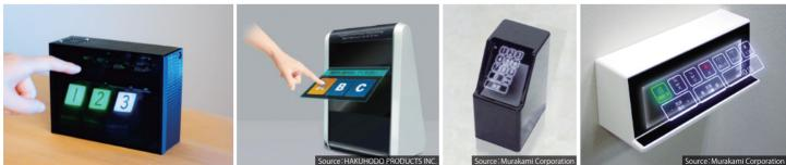
Touchless user interface system : By combining the "Floating Image" and sensing technologies, our floating touch panel and air switch devices can be operated without physically touching anything.
