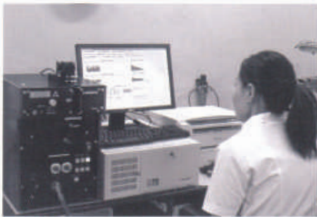
Complete apparatus of Japanese advanced "laserspot -V" is used to define the quality of hairiness and thickness of the yarn count.
