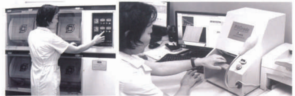
Pill Grade complete apparatus, manufactured in Japan is used to determine fill notes of woven and knitted finished products.
