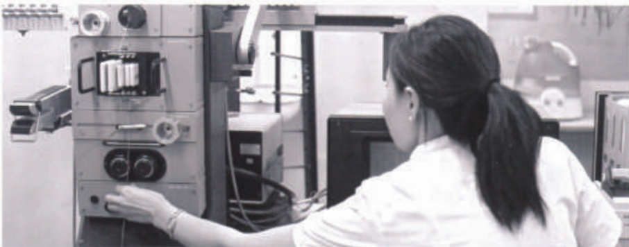
Yarn breaking force and elongation determination of Japanese "TENSILE TESTING MACHINE VS -200 automatic device.
