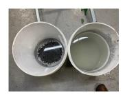
cyclone separation, improved with our original technology, removes 99.9% of sludge just by spiraling flow<sup>1</sup>. This remarkably reduces clogging of the filter. Moreover, it is possible to use only the main unit, cyclone separator that removes sludge from industrial wastewater without a filter. Therefore, Three Zeroes is possible: zero running cost, zero industrial waste, and zero maintenance.
