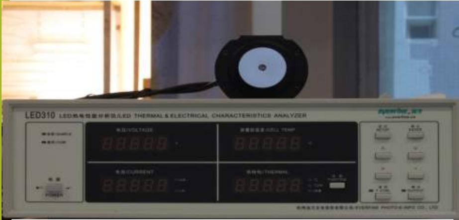
LED thermal resistance & Junction temperature testing
