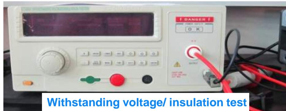
Withstanding voltage/ insulation test
