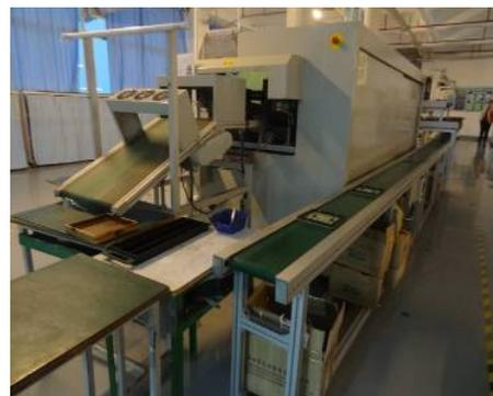
Wave solder carrier return automation
